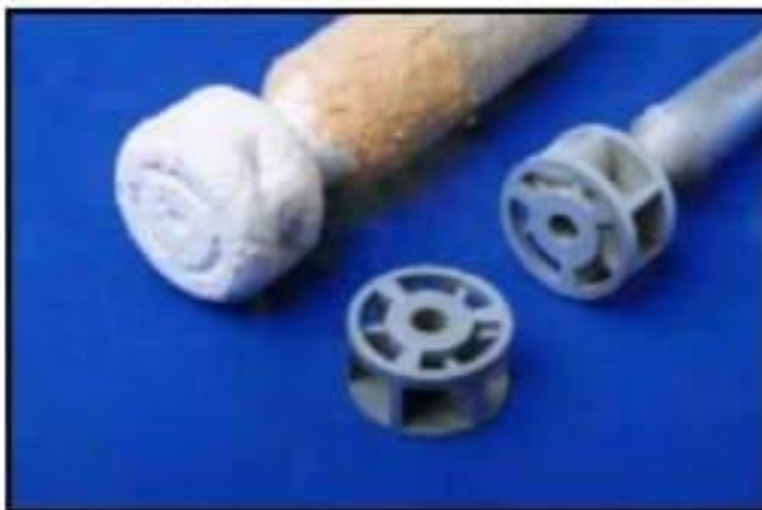
SLS-produced investment casting shell for impeller wheel (source: Fraunhofer Institute IPT)
